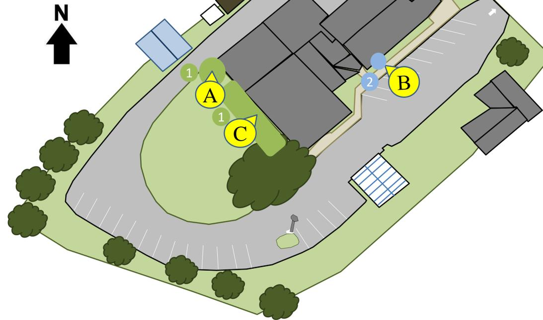
**1 BIORETENTION SYSTEM:** A bioretention system could be installed near the northwestern corner of the building where downspouts drain into the grass as well as along the western side of the building. A bioretention system will reduce runoff and allow stormwater infiltration, decreasing the amount of contaminants that reaches catch basins.
